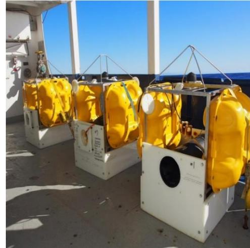
Seafloor pressure sensors measure cm-level vertical movement of the seafloor during slow slip events and earthquakes, and can also detect passing tsunami waves
