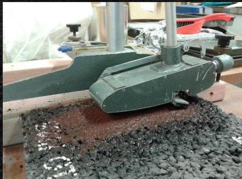
*Pendulum skid resistance testing*
