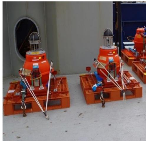
Seafloor transponders enable tracking of horizontal motions of the seafloor over time (at mm to cm level)
