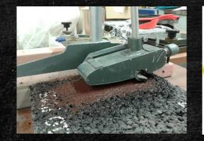
Pendulum skid resistance testing
