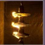
3 mm of ash fall cover on a glass insulator string inducing a flashover. Note how the current is tracking through the volcanic ash covered insulator surface
