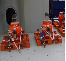
Seafloor pressure sensors measure cmlevel vertical movement of the seafloor during slow slip events and earthquakes, and can also detect passing tsunami waves
