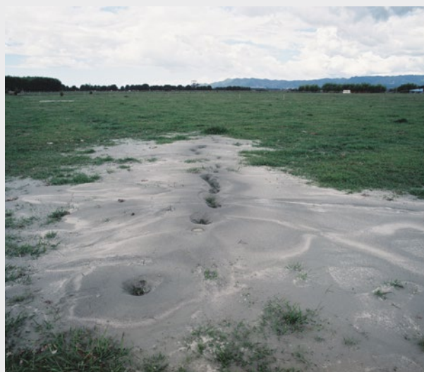
Sand boils and liquefaction after Edgecumbe Earthquake, 2 March 1987. Source: GNS Science Photographer: Lloyd Homer
